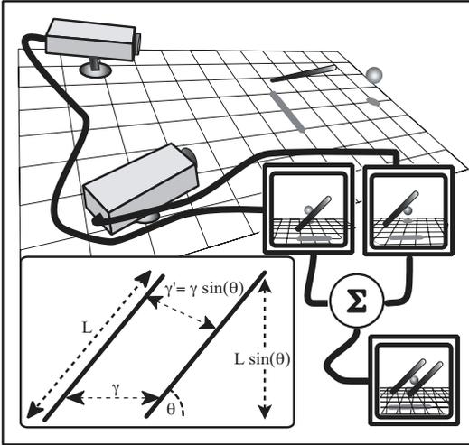
Figure 2. Two cameras record slightly different views of a rod (oriented at  $\theta^\circ$  with respect to horizontal) when focusing on the more distant sphere. Summing the images produces the double image of the rod. The insert shows the length of the rod,  $L$ , the vertical projection of the rod ( $L \sin \theta$ ), the horizontal separation of the double rod images ( $\gamma$ ), and their perpendicular separation ( $\gamma \sin \theta$ ).
