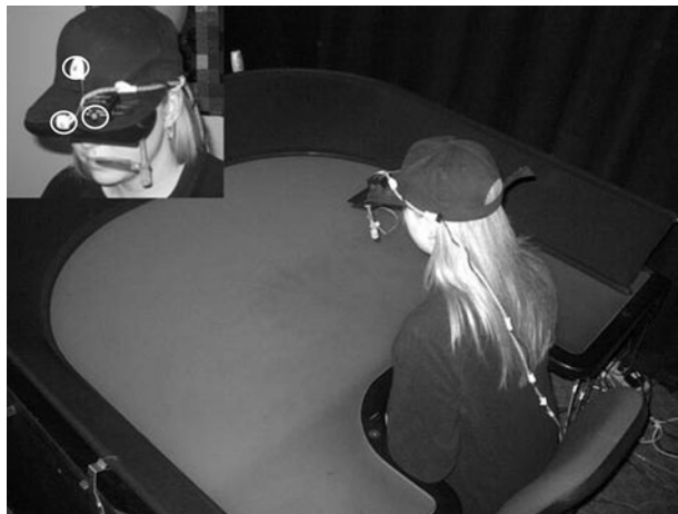
Figure 1. A photograph of a research participant wearing the head-mounted eyetracking unit and seated at a display table used in the experiments in our lab. Inset: Frontal view of the eyetracker with the attached infrared-emitting diodes (IREDs, circled in white) used to track movements of the head.
