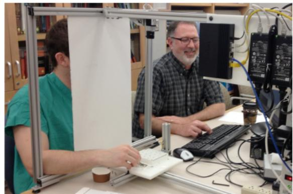
Figure 1. Box skills trainer. A resident trainee places a peg on the horizontal pegboard. The proctor updates video images, visible on a display located behind the keyboard.
