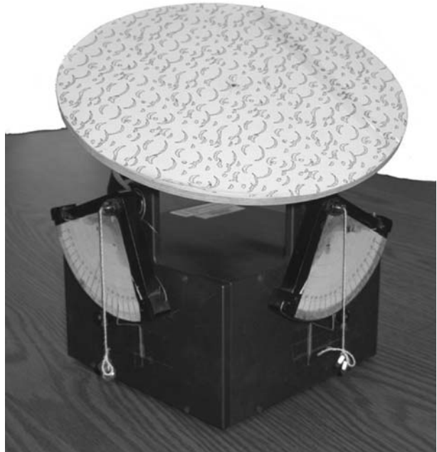
Fig. 8 The slope indicator. The circular top surface rotates about a pivot point below its center
