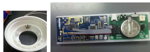
Figure 2: The microswitch mounted inside the cap (left). The electronics including the TelosB mote and custom board with button cell battery at right.
