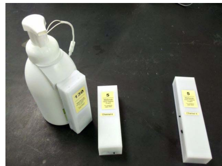
Figure 1: From left to right, the dispenser, receiver and transmitter.
