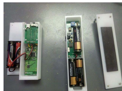
Figure 3: The door minder. The receiver is on the left with the mote (bottom), circuit board (top) and two batteries mounted on the case lid. The transmitter is on the right, with 3 AA batteries and a strip of adhesive magnetic tape on its lid.
