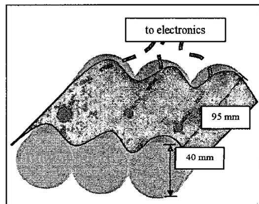
Figure 1. Training setup (3 silicone cylinders with embedded polyethylene balloons with filler tubes leading to the electronic filling and sensing device)
